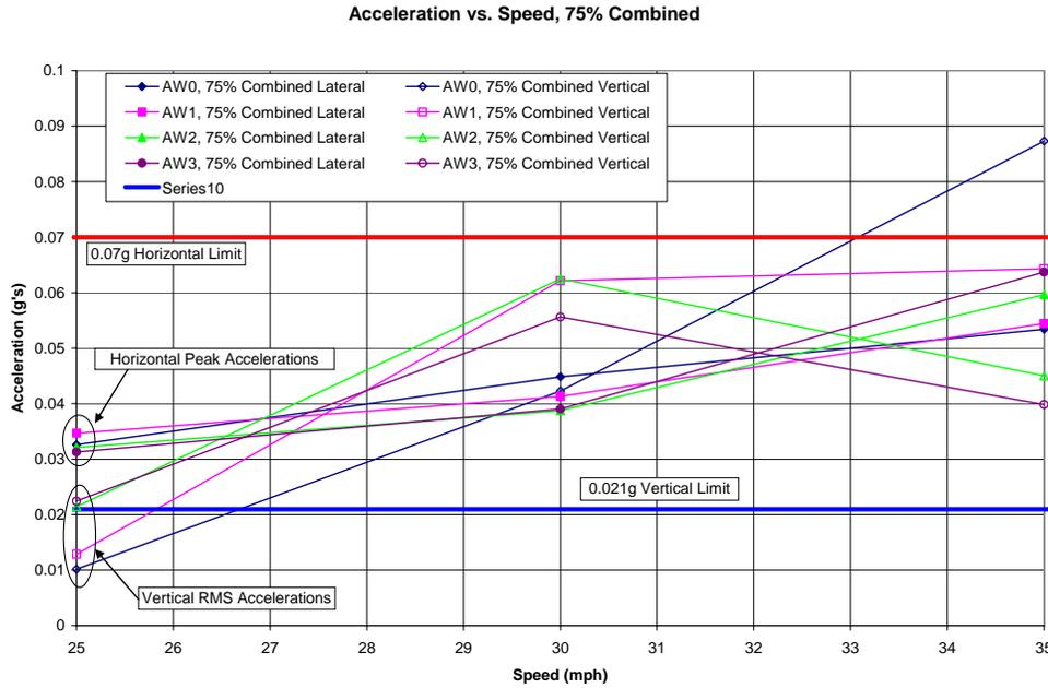
**Figure 3-17: RMS Vertical and Peak Horizontal Acceleration with 1.65° Vertical and 0.825° Horizontal Rotation at Joint.**
