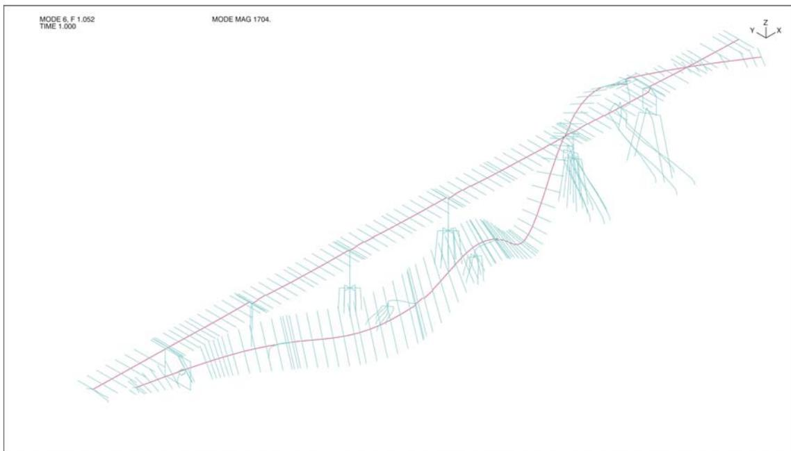
**Figure 3-41: Mode Shape 6 (Vertical Line L – Period = 0.95 sec)**
