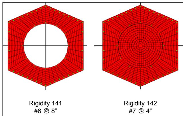
Figure 3-25: LM Pier 4 – SPERC Model
