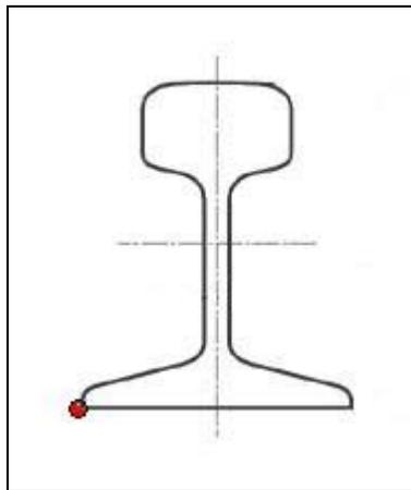
**Figure 3-27: Rail Cross-Section – Point of Maximum Normal Stress**
