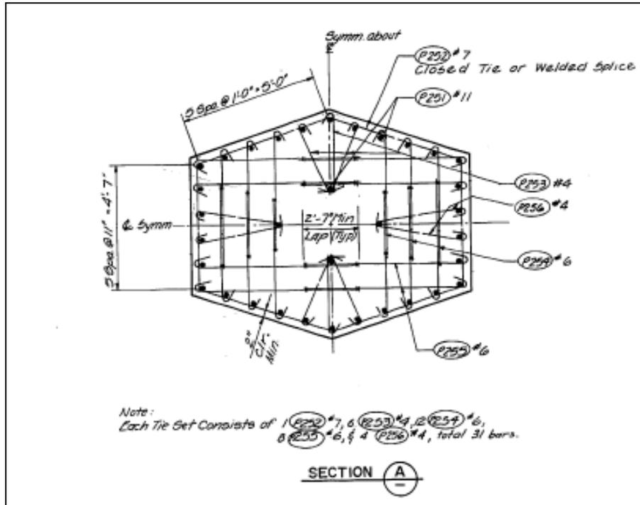
Figure 3-20: LM Pier 2 – drawing 304
