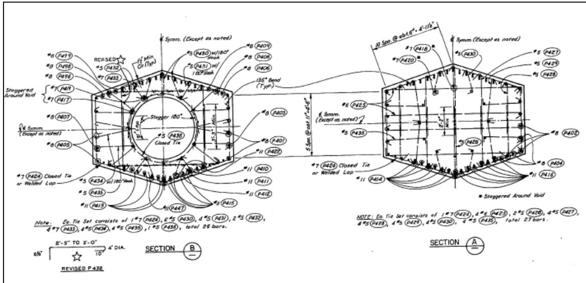
Figure 3-12: LL Pier 4 Column Reinforcement - drawing 292
