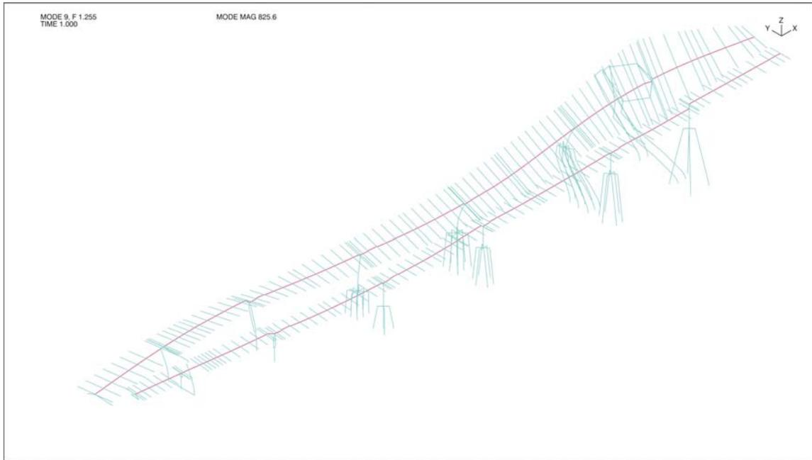
**Figure 3-44: Mode Shape 9 (Transverse Line L – Period = 0.80 sec)**
