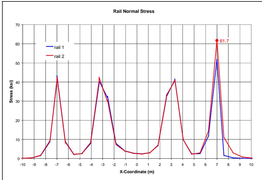
**Figure 3-25: Combined Maximum Vertical (YY) and Lateral (ZZ) Rotation – Rail Normal Stress (ksi).**
