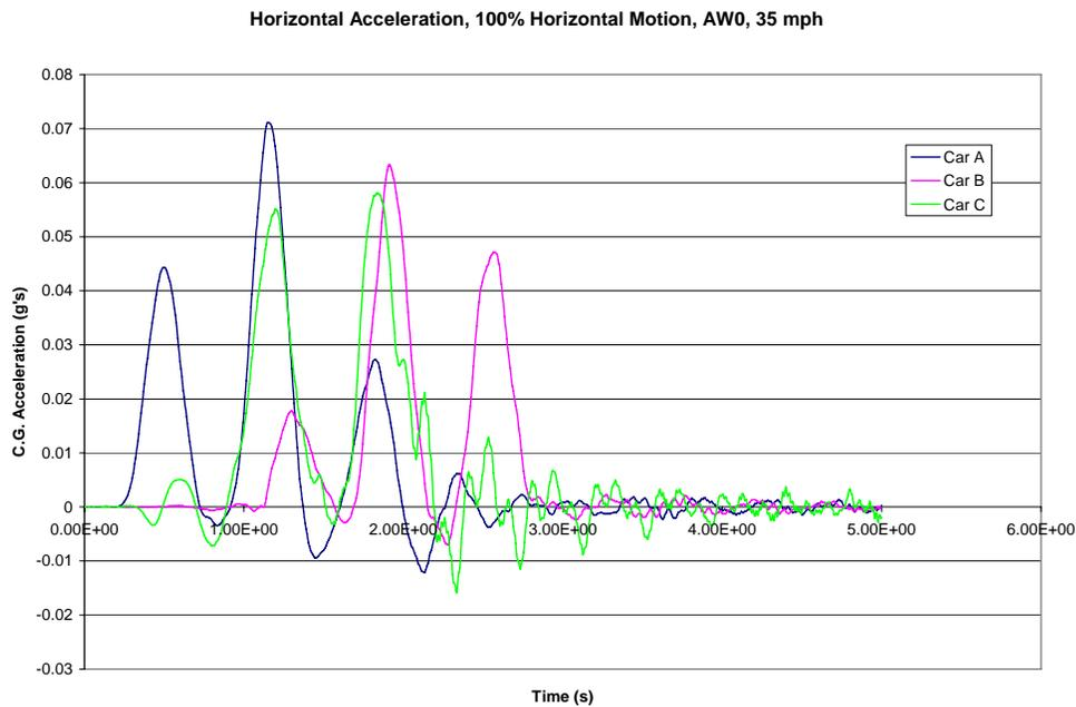
**Figure 3-11: Lateral acceleration with 1.1° horizontal rotation at joint**
