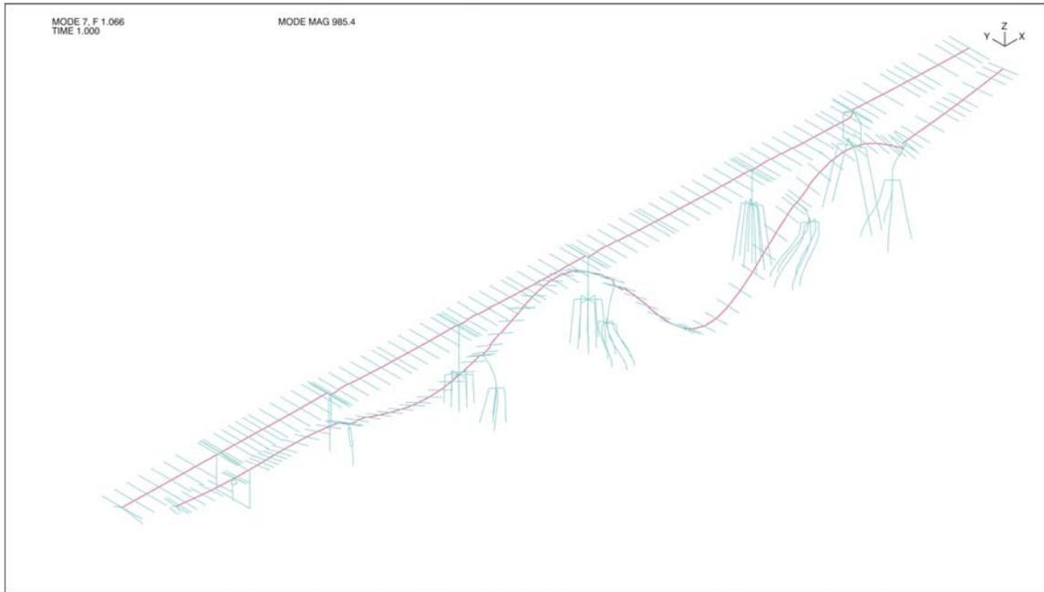
**Figure 3-42: Mode Shape 7 (Vertical Line M – Period = 0.94 sec)**
