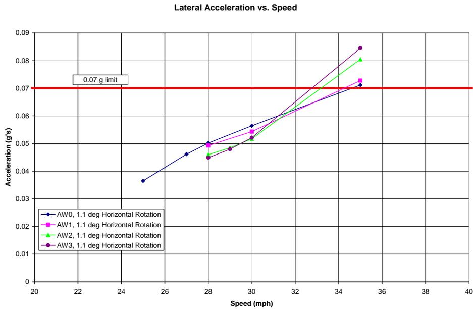
Figure 3-12: Peak Horizontal Acceleration vs. Speed, 100% Horizontal Rotation
