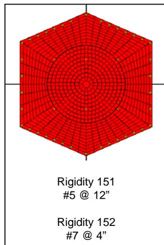
**Figure 3-27: LM Pier 5 – SPEMC Model**
