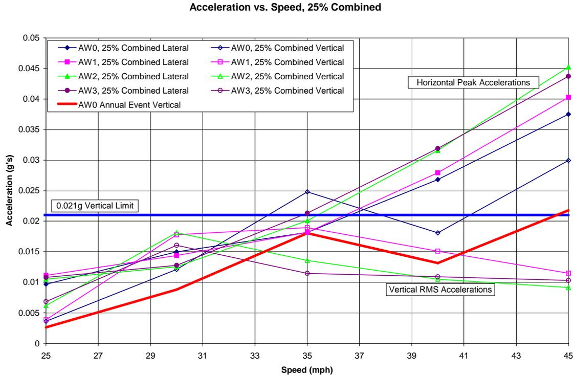
**Figure 3-19: RMS Vertical and Peak Horizontal Acceleration with 0.55° Vertical and 0.275° Horizontal Rotation at Joint.**
