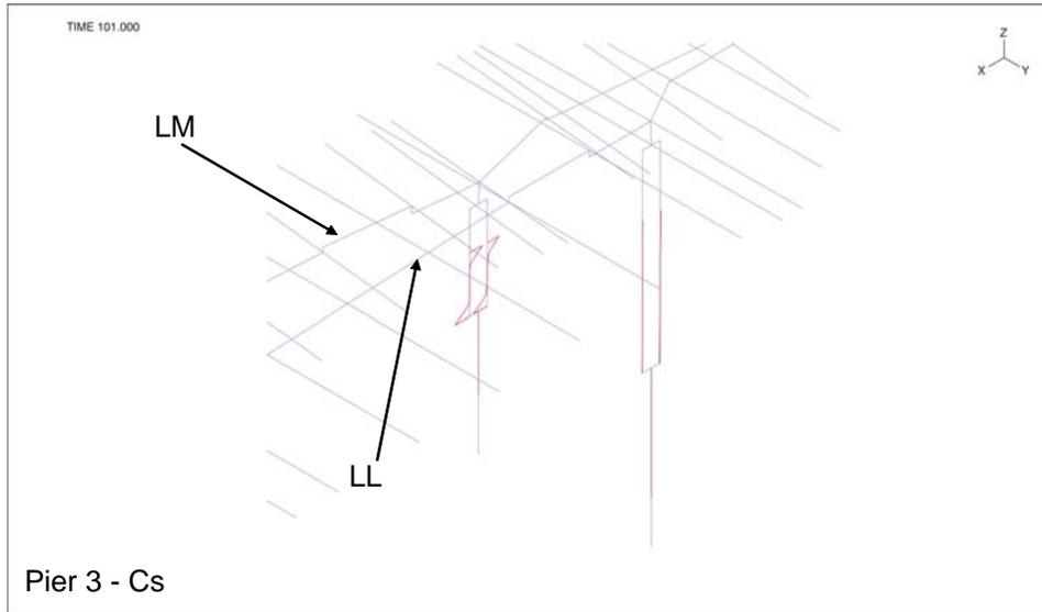
**Figure 3-51: Plastic Curvature about Transverse Axis (S-axis) – Pier 3**
