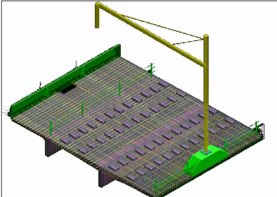
**Figure 2-1: Two-Track OCS Cantilever Structure (Parsons and INCA [1])**
