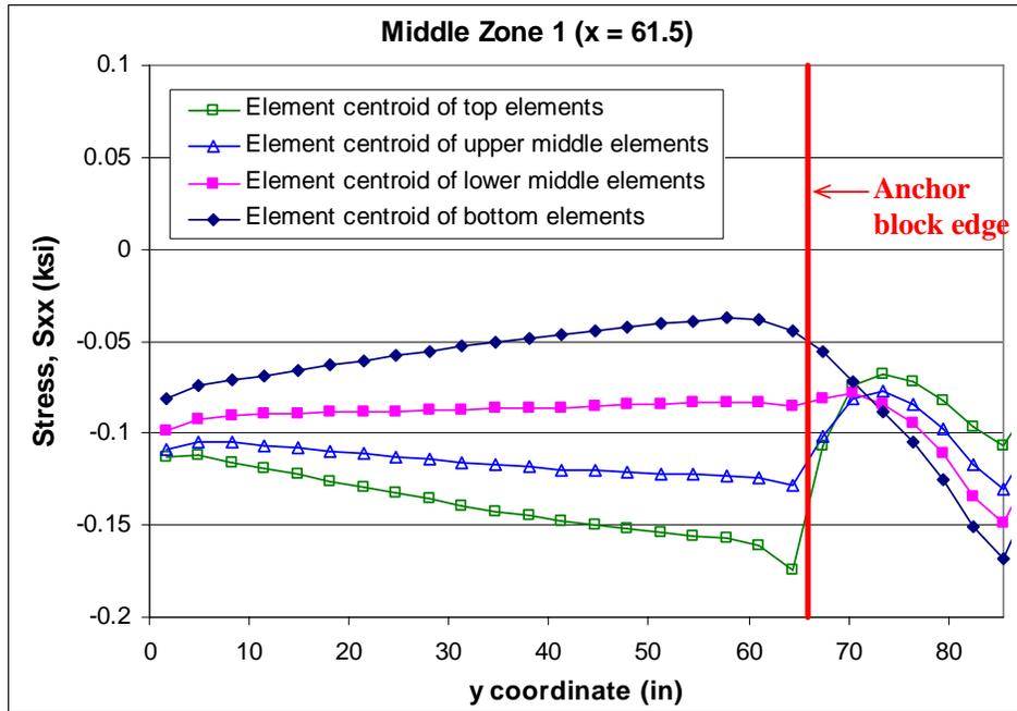
**Figure 3-3: Longitudinal Stress (Sxx) Variation in the y-direction**
