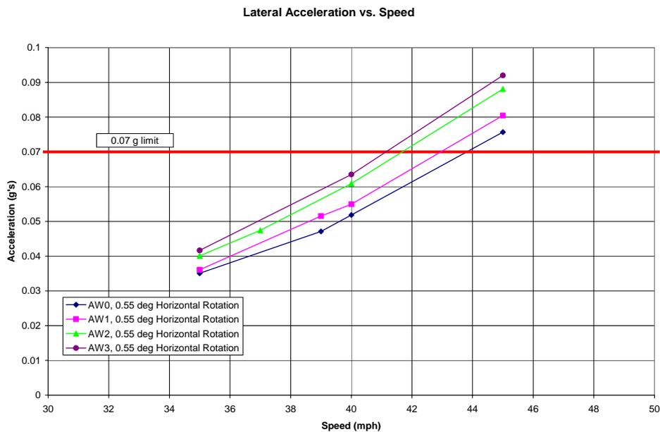
Figure 3-13: Peak Horizontal Acceleration vs. Speed, 50% Horizontal Rotation.
