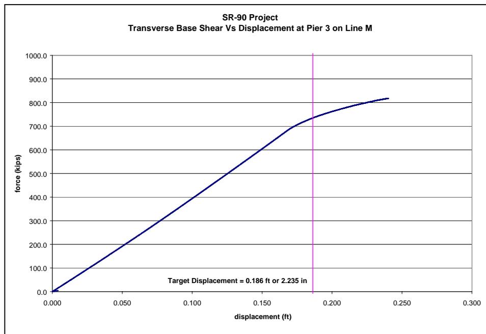
**Figure 3-69: Column Force vs. Displacement at Pier 3 on Line M**
