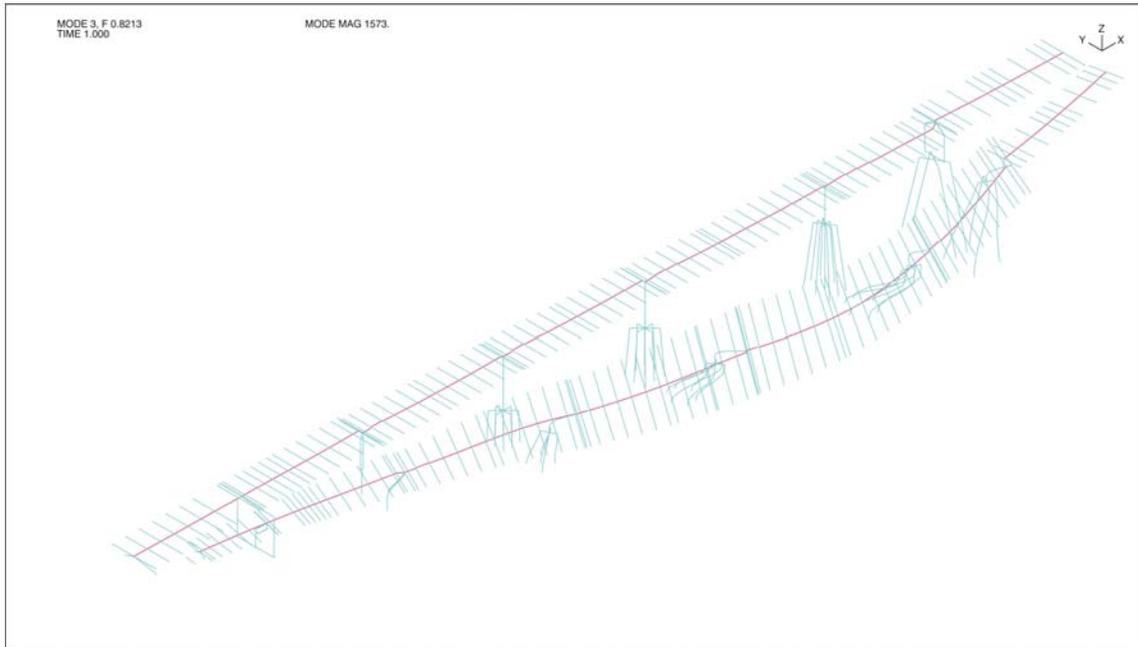
**Figure 3-38: Mode Shape 3 (Transverse Line M – Period = 1.22 sec)**
