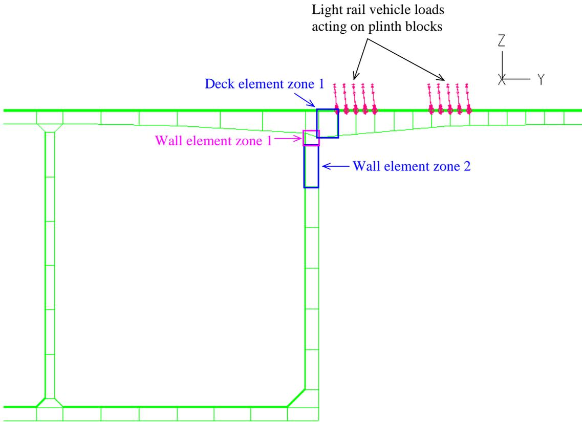
**Figure 3-5: Critical Zones selected for Stress Investigation – Elevation View**
