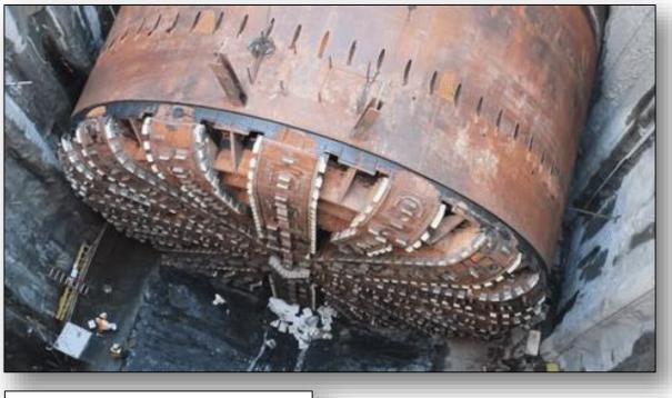
Testing the cutterhead rotation
