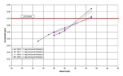
Figure 3-12: Peak Horizontal Acceleration vs. Speed, 100% Horizontal Rotation
