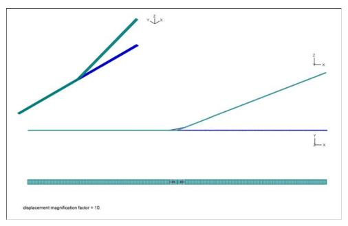
Figure 3-10: Maximum Vertical (YY) Rotation – Deformed Mesh.
