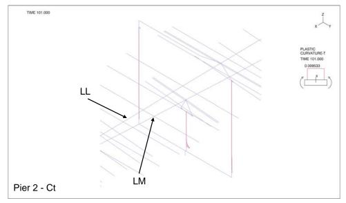
Figure 3-50: Plastic Curvature about Longitudinal Axis (T-axis) – Pier 2
