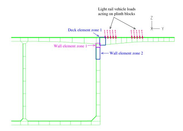
**Figure 3-5: Critical Zones selected for Stress Investigation – Elevation View**
