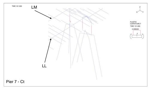
Figure 3-59: Plastic Curvature about Longitudinal Axis (T-axis) – Pier 7
