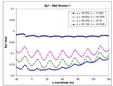
Figure 3-7: Principal Tensile Stress Variation in the x-direction at Wall Section 1 – Self Weight +Post Tension Forces +Light Rail Vehicle Loads +OCS Loads (Case 1)
