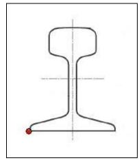
Figure 3-27: Rail Cross-Section – Point of Maximum Normal Stress
