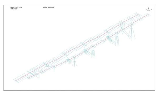
Figure 3-36: Mode Shape 1 (Longitudinal Line L – Period = 1.73)
