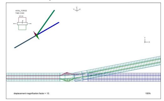
Figure 3-20: Combined Maximum Vertical (YY) and Lateral (ZZ) Rotation – Rail Axial Force on Deformed Mesh.
