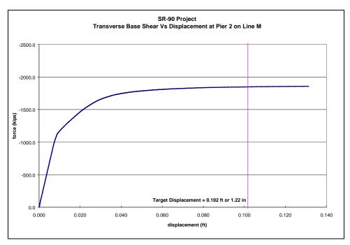
Figure 3-68: Column Force vs. Displacement at Pier 2 on Line M
