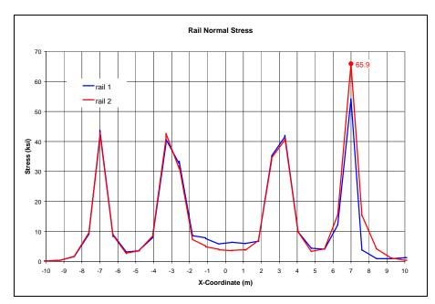
Figure 3-34: Combined Maximum Vertical (YY) and Lateral (ZZ) Rotation – Rail Normal Stress Envelope (ksi).
