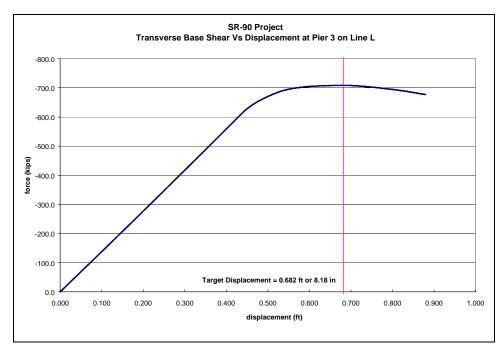
Figure 3-62: Column Force vs. Displacement at Pier 3 on Line L
