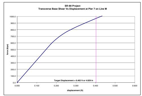
Figure 3-73: Column Force vs. Displacement at Pier 7 on Line M
