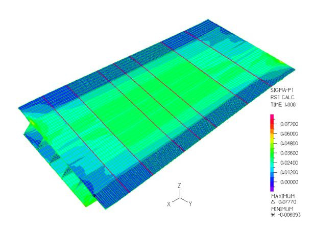
Figure 3-3: Principal Tensile Stress (Sp1) Contour Plot under a Torsion of 6202 kipft
