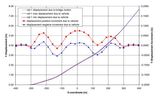
Figure 3-30: Rail Lateral (Y) Displacements due to Joint Lateral (ZZ) Rotation and Wheel Reactions.
