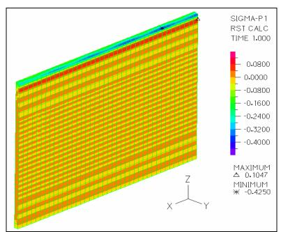
Figure 3-16: Principal Tensile Stress Contour Plot at the Outer Surface of the Wall – Self Weight +Post Tension Forces +Light Rail Vehicle Loads+OCS Loads (Case 1)
