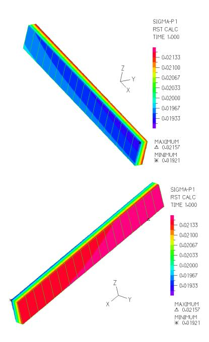
Figure 3-10: Principal Tensile Stress (Sp1) Contour Plots at the Wall Element Zone 2 under a Torsion of 6202 kip-ft
