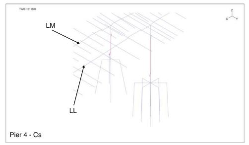
Figure 3-52: Plastic Curvature about Transverse Axis (S-axis) – Pier 4
