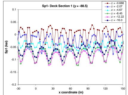
Figure 3-13: Principal Tensile Stress (Sp1) Variation in the x-direction at Deck Section 1 - Self Weight + Post Tension Forces + Light Rail Vehicle Loads (Case 2)
