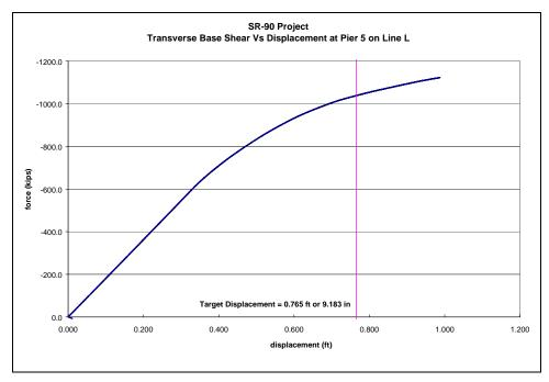
Figure 3-64: Column Force vs. Displacement at Pier 5 on Line L
