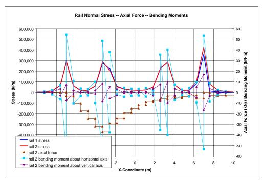
Figure 3-26: Combined Maximum Vertical (YY) and Lateral (ZZ) Rotation – Rail Normal Stress (kPa) – Axial Force (kN) – Bending Moments (kN-m).
