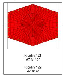
Figure 3-21: LM Pier 2 – SPEMC Model
