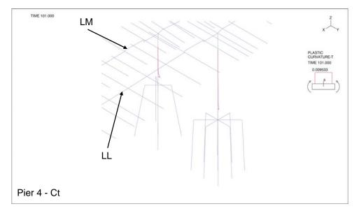
Figure 3-53: Plastic Curvature about Longitudinal Axis (T-axis) – Pier 4
