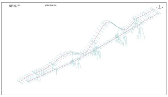
Figure 3-43: Mode Shape 8 (Torsion-Transverse Line M – Period = 0.93 sec)
