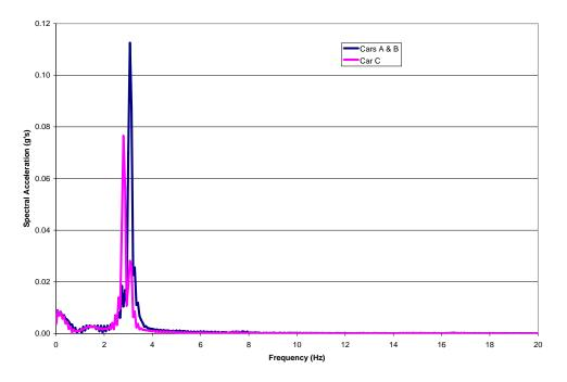
Figure 3-10: Vertical Spectral Acceleration, 35 mph, AW0
