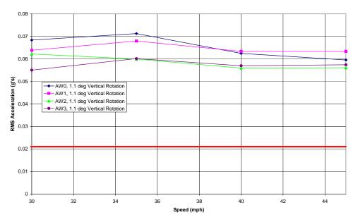
Figure 3-15: RMS Vertical acceleration with 1.1° vertical rotation at joint.
