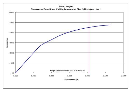
Figure 3-60: Column Force vs. Displacement at Pier 2 (North Column) on Line L
