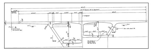
Figure 3-33: Typical Superstructure Cross-Section
