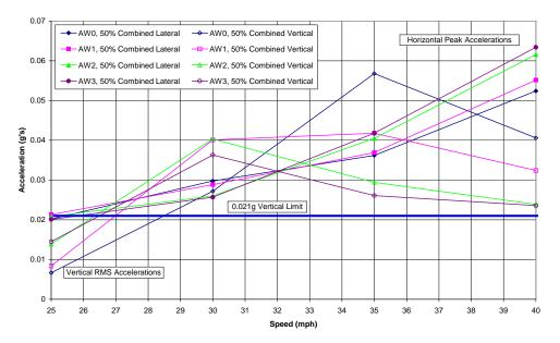
Figure 3-18: RMS Vertical and Peak Horizontal Acceleration with 1.1° Vertical and 0.55° Horizontal Rotation at Joint.
