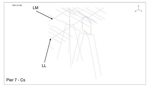
Figure 3-58: Plastic Curvature about Transverse Axis (S-axis) – Pier 7
