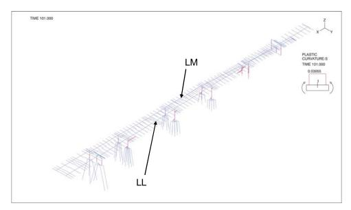
Figure 3-47: Plastic Curvature about Transverse axis (S-axis) at the Target Displacement
