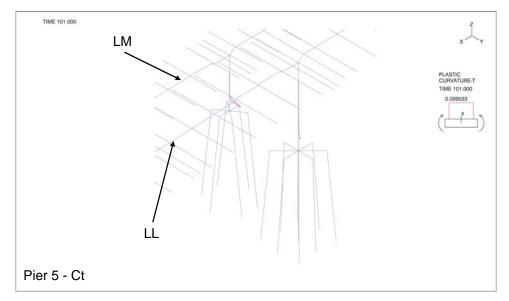
Figure 3-55: Plastic Curvature about Longitudinal Axis (T-axis) – Pier 5
