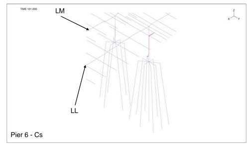
Figure 3-56: Plastic Curvature about Transverse Axis (S-axis) – Pier 6
