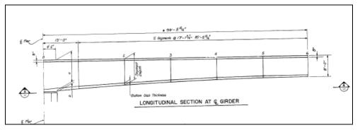
Figure 3-34: Variation in Depth for Cross-Sections along a Typical Span.
