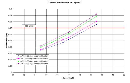
Figure 3-13: Peak Horizontal Acceleration vs. Speed, 50% Horizontal Rotation.
