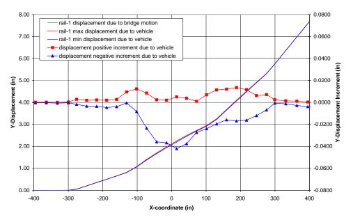
Figure 3-32: Rail Lateral (Y) Displacements due to Joint Combined Lateral (ZZ) and Vertical (YY) Rotation and Wheel Reactions.
