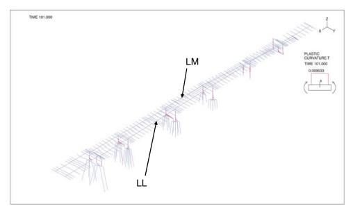
Figure 3-49: Plastic Curvature about Longitudinal axis (T-axis) at the Target Displacement
