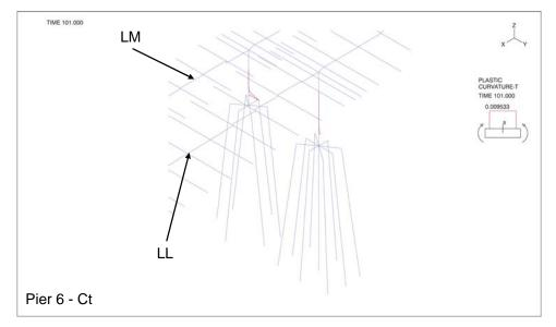
Figure 3-57: Plastic Curvature about Longitudinal Axis (T-axis) – Pier 6
