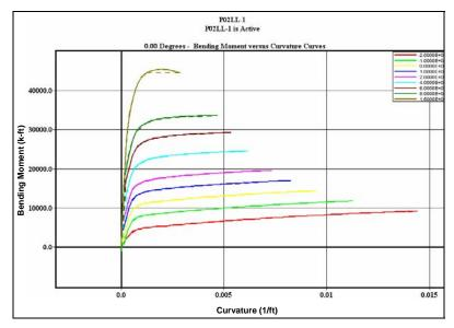
Figure 3-32Typical Moment-Curvature Relation of Piers
