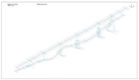
Figure 3-39: Mode Shape 4 (Longitudinal Line M -- Period = 1.17 sec)
