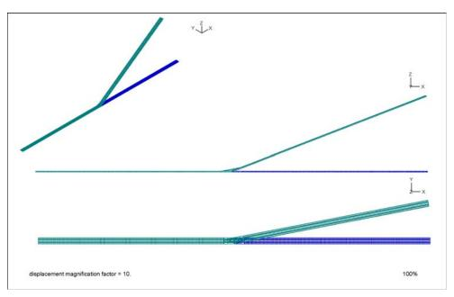
Figure 3-12: Combined Maximum Vertical (YY) and Lateral (ZZ) Rotation – Deformed Mesh.
