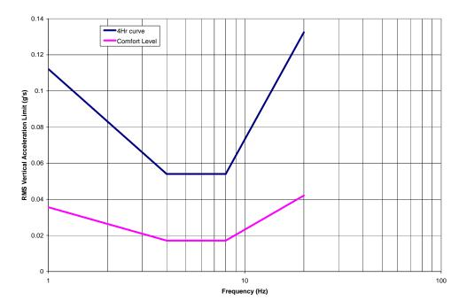
**Figure 3-9: Reformatted Vertical Acceleration Limits**
