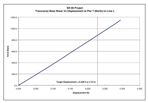
Figure 3-66: Column Force vs. Displacement at Pier 7 (North Column) on Line L
