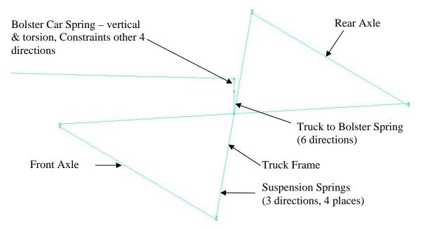
Figure 3-4: Truck B Detail
