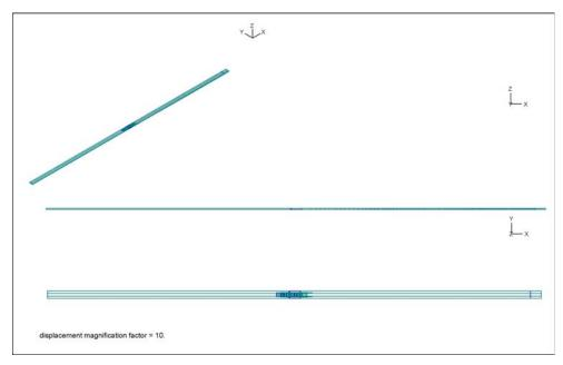
Figure 3-9: Maximum Longitudinal (X) Translation – Deformed Mesh.
