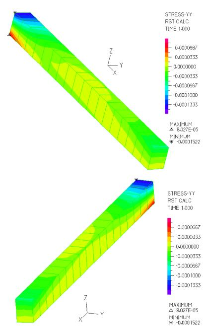
Figure 3-7: Transverse Normal Stress (Syy) Contour Plots at the Deck Element Zone 1 under a Torsion of 6202 kip-ft
