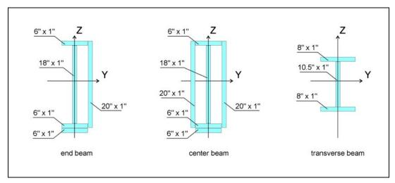
**Figure 3-7: Expansion Joint Model – Three-Beam Transition System Element Cross-Sections – Dimensions in Inches.**
