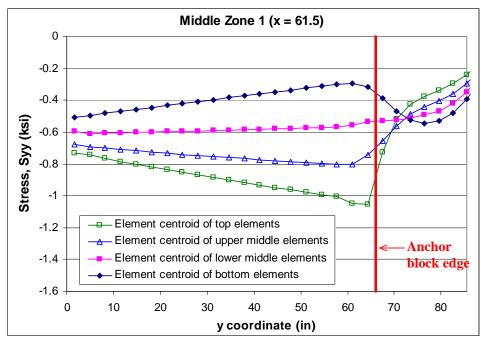
Figure 3-2: Transverse Stress (Syy) Variation in the y-direction
