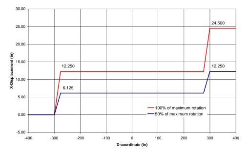
Figure 3-16: Rail Longitudinal (X) Displacements due to Joint Longitudinal (X) Translation.
