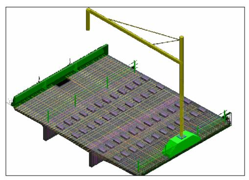
Figure 2-1: Two-Track OCS Cantilever Structure (Parsons and INCA [1])
