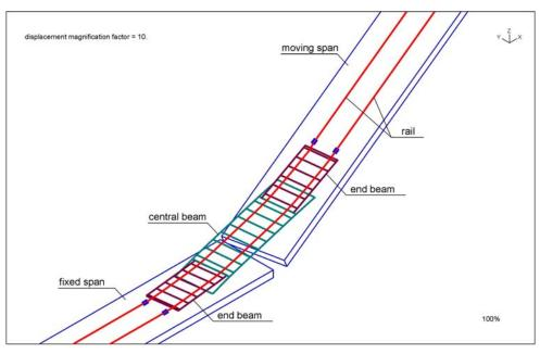
Figure 3-19: Deformed Expansion Joint Model Details.
