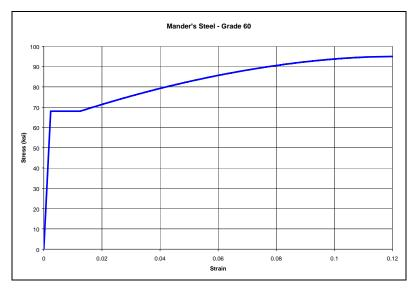
Figure 3-6: Typical Steel Stress-Strain Relation
