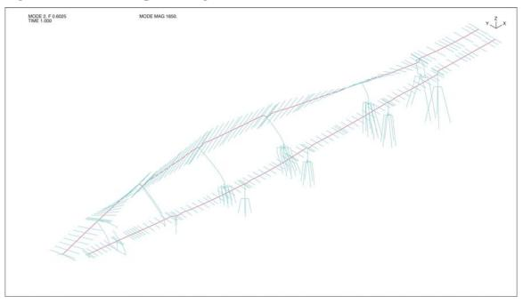
Figure 3-37: Mode Shape 2 (Transverse Line L – Period = 1.66 sec)
