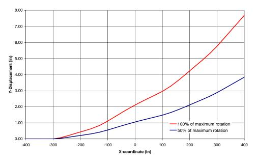
Figure 3-18: Rail Lateral (Y) Displacements due to Joint Lateral (ZZ) Rotation.
