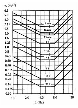
**Figure 3-8: Vertical Acceleration Limits**
