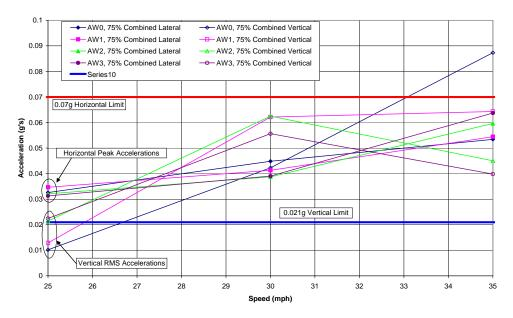
Figure 3-17: RMS Vertical and Peak Horizontal Acceleration with 1.65° Vertical and 0.825° Horizontal Rotation at Joint.
