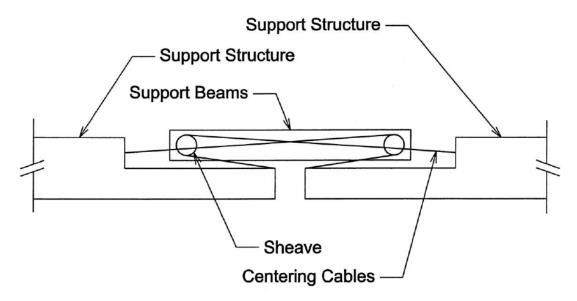
Figure 3-4: Cable System for Centering the Track Bridge (from [1])
