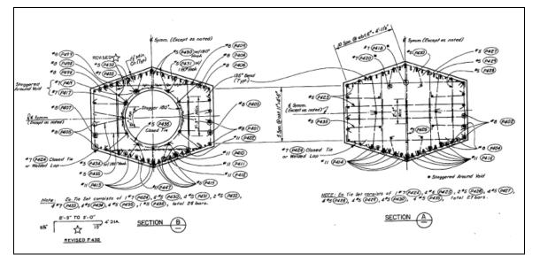
Figure 3-12: LL Pier 4 Column Reinforcement - drawing 292
