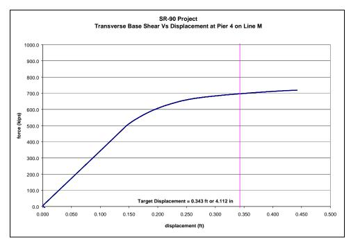
Figure 3-70: Column Force vs. Displacement at Pier 4 on Line M
