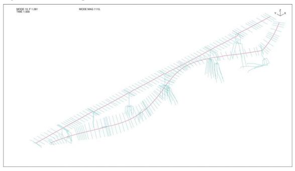
Figure 3-45: Mode Shape 10 (Transverse Line M – Period = 0.78 sec)
