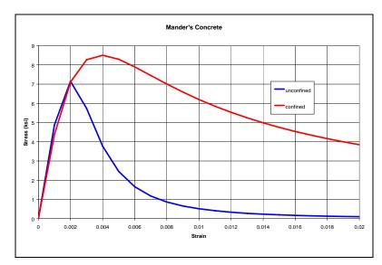
Figure 3-7: Typical Concrete Stress-Strain Relation
