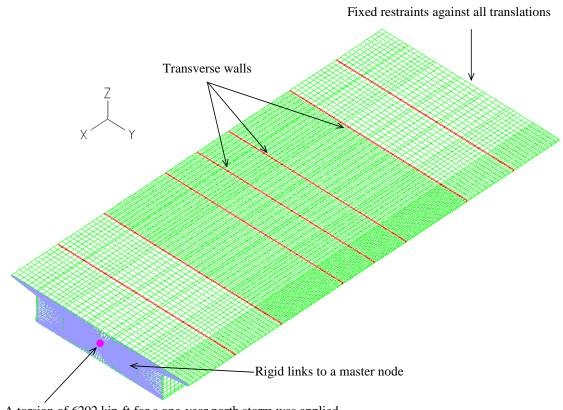
A torsion of 6202 kip-ft for a one-year north storm was applied to a master node at the centroid of the end section
