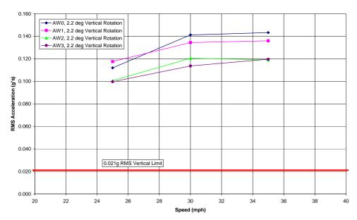
Figure 3-14: RMS Vertical acceleration with 2.2° Vertical rotation at joint
