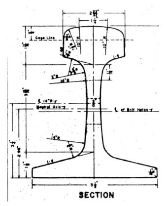
Figure 3-8: 115 LB RE Rail, Cross Section, Dimensions in Inches.
