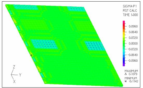
Figure 3-17: Principal Tensile Stress Contour Plot at the Top Surface of the Deck – Self Weight + Post Tension Forces + Light Rail Vehicle Loads +OCS Loads (Case 1)
