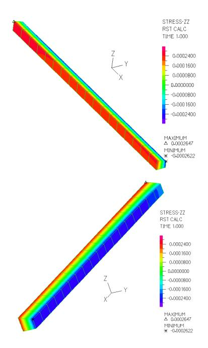
Figure 3-9: Vertical Normal Stress (Szz) Contour Plots at the Wall Element Zone 1 under a Torsion of 6202 kip-ft
