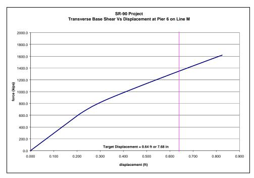
Figure 3-72: Column Force vs. Displacement at Pier 6 on Line M
