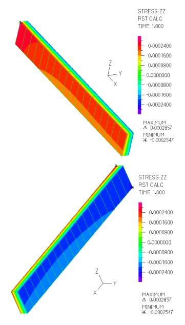
Figure 3-11: Vertical Normal Stress (Szz) Contour Plots at the Wall Element Zone 2 under a Torsion of 6202 kip-ft
