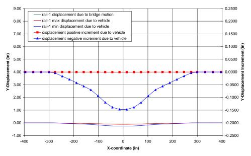
Figure 3-31: Rail Vertical (Z) Displacements due to Joint Lateral (ZZ) Rotation and Wheel Reactions.
