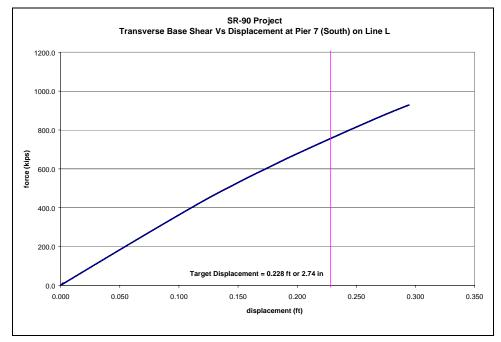
Figure 3-67: Column Force vs. Displacement at Pier 7 (South Column) on Line L
