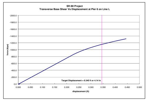
Figure 3-65: Column Force vs. Displacement at Pier 6 on Line L
