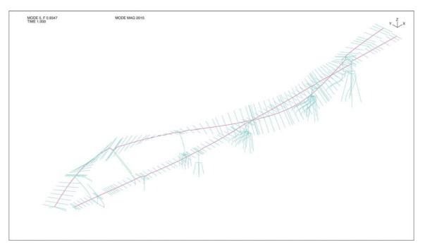
Figure 3-40: Mode Shape 5 (Transverse Line L – Period = 1.07 sec)
