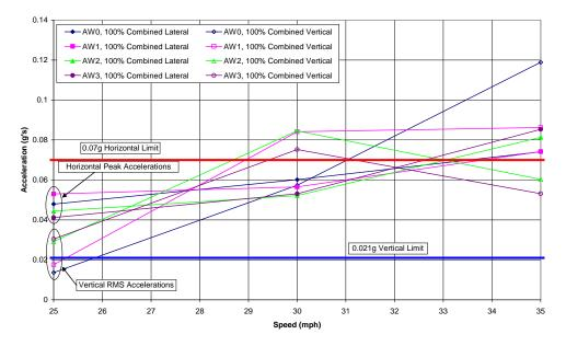
Figure 3-16: RMS Vertical and Peak Horizontal Acceleration with 2.2° Vertical and 1.1° Horizontal Rotation at Joint.
