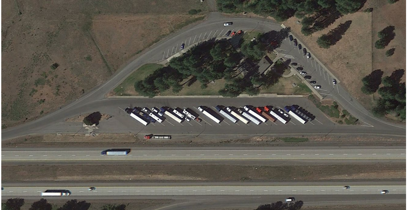
Figure 2.5 Herringbone Drive-Through Slots at Interstate Rest Area
