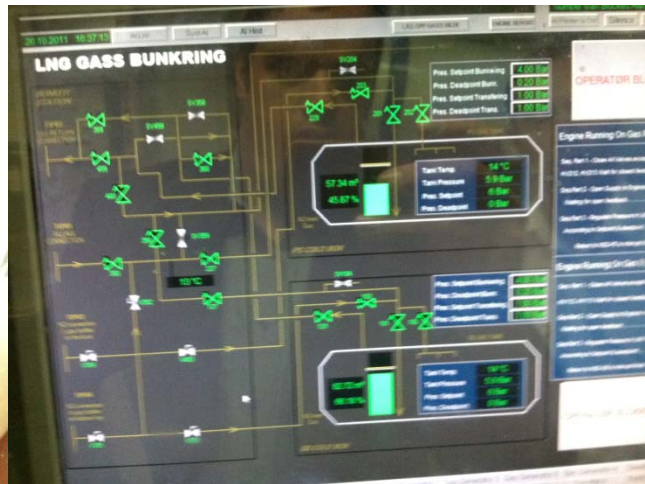
Oiler (blue glove) Measuring diesel tank aboard WSF with measuring stick (left) and measurement system for LNG on Tide Sjo passenger vessel (right) that monitors whole system for pressure and potential leaks
