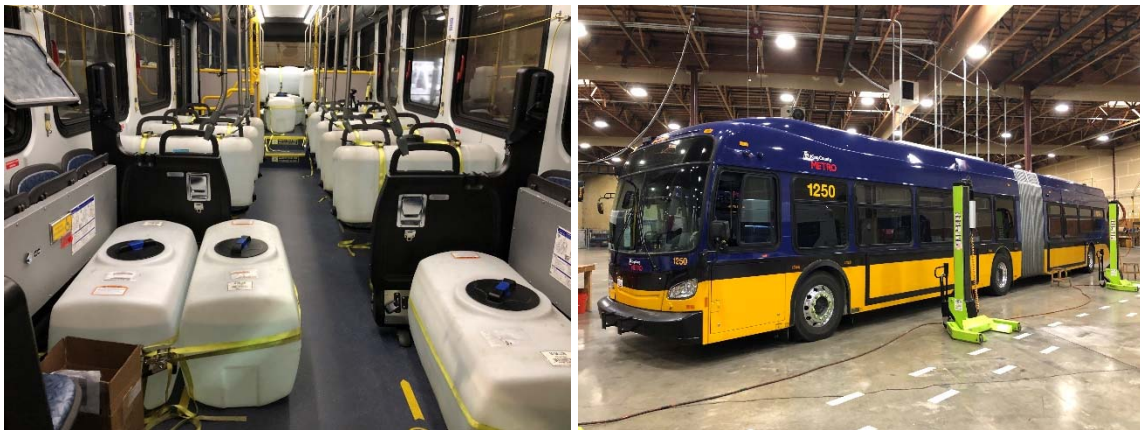
Left to right: A Proterra battery-electric bus with onboard water to simulate passenger loads; A New Flyer battery-electric articulated bus.
