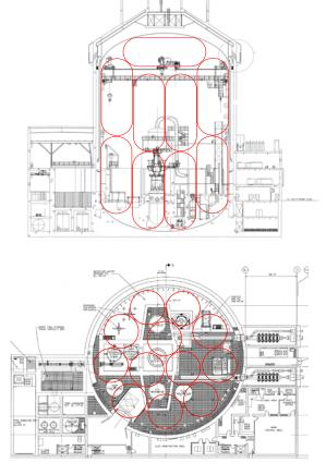
25 Westinghouse SMR Containment Vessels fit into single AP1000 Containment Vessel
