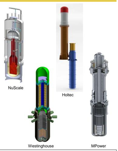
These LW-based designs are considered Integral Pressurized Water Reactor (IPWR) Designs
