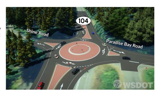
to accommodate the largest legal loads on a highway, including semis. The final design recommendations will include splitter islands and truck aprons with rolled-curbing similar to what was constructed last summer at SR 20 and Sharpes Corner in Anacortes which is
