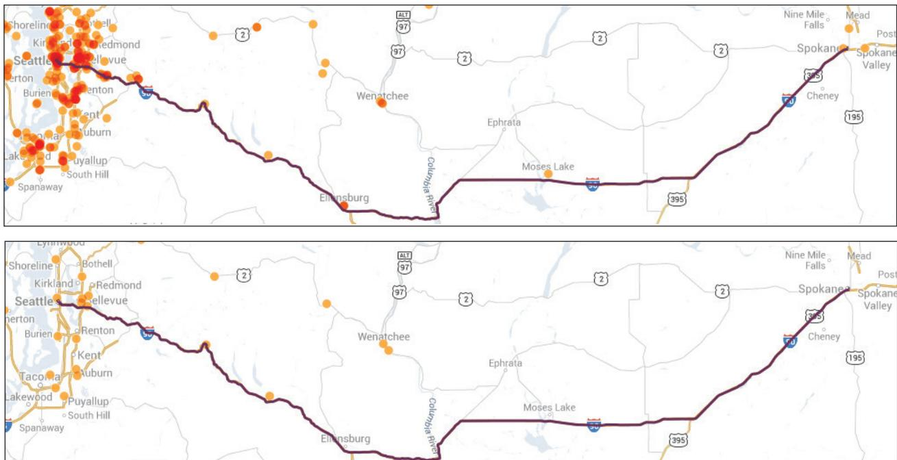
**The high concentration of publicly available charging locations along the western segment of the route enables easy BEV travel.** There are 12 DC fast charging locations and 210 Level 2 charging locations in and around Seattle. All BEVs in the simulations were able to travel the western segment of the route without the vehicles' battery reaching a 20 percent state of charge.
