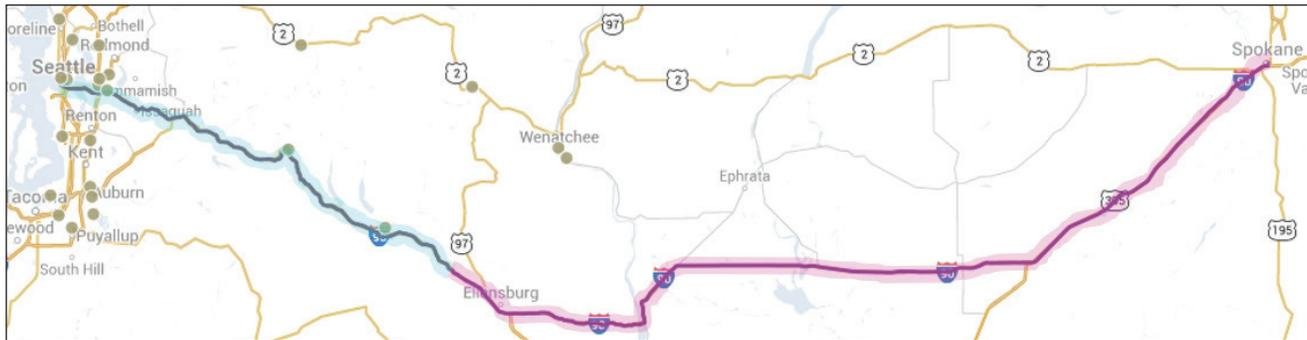
Tan circles (●) indicate locations of existing DC fast charging stations. Lengths of road highlighted in cyan (—) indicate sections along the route where BEV travel is currently possible using existing publicly accessible DC fast charging stations. Lengths of road highlighted in magenta (—) indicate sections along the route where BEV travel is currently not possible using existing publicly accessible DC fast charging stations.
