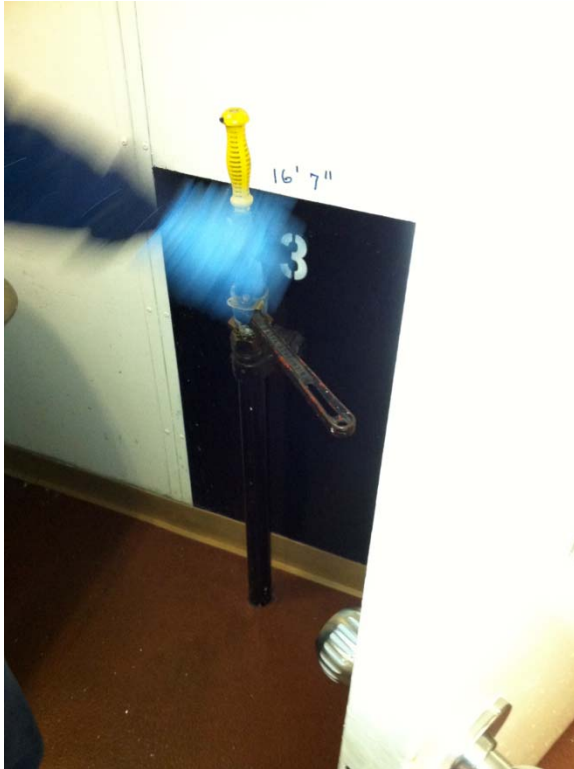
Oiler (blue glove) Measuring diesel fuel tank level aboard WSF with measuring stick (left) and measurement system for LNG on Fjord1 vessel (right) that monitors whole system for pressure and potential leaks
