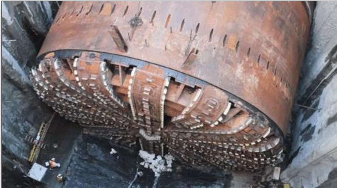
*Testing the cutterhead rotation*
