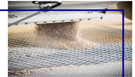
Gravity pit unloading
